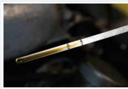
Checking the oil level and condition
