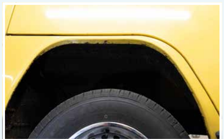
Front arch rust
